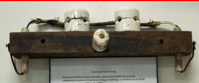
Knob & Tube wiring can still be found in some of the older homes in Tallahassee.
