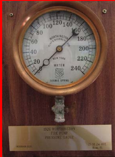
Pressure gauge off a 1926 manually operated Worthington Fire Pump. It is from the Ingram building in downtown Miami. Pump had to be changed out because it was not automatic.
